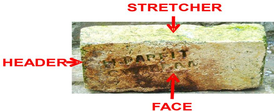
The two large surfaces, the back and front, are referred to as "faces", the long sides as "stretchers", and the ends as "headers".
